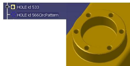
Figure 29. Data conversion software infers a hole-pattern feature from the geometry.
